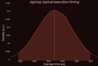
The timing distribution of signature generation from an arbitrary byte array on BN\_254, yielding an average runtime of  $954 \pm 7\mu s$ .
